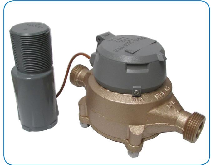
Endpoints also support collection of a current endpoint reading, status indicators and snapped daily read (midnight UTC) for mobile (walk-by or drive-by) data collection. Using the two-way endpoint feature, historical interval data and other endpoint information can be captured from the endpoint during the mobile reading process.
